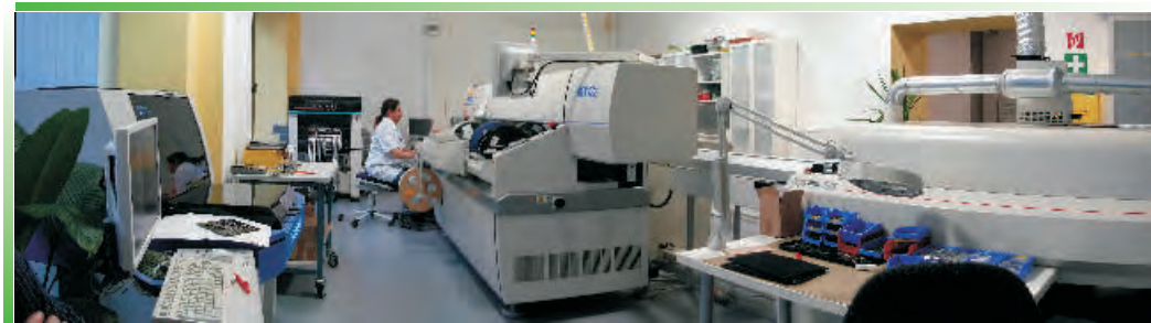
ZIMO production machine room: two placement robots, Reflow soldering oven, soldering-paste printer, AOI device.
